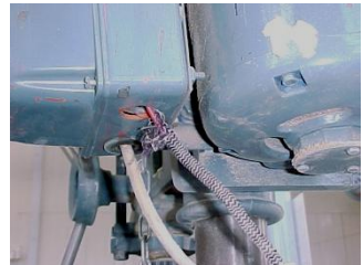
Exposed cables on a drill press
