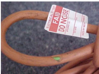
Visual damage to an extension lead
